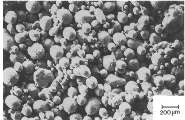
Figure 2 (b) Prealloyed NiAl powder. After 20 min of mechanofusion, the particles became spherical and displayed a finer particle size (SEM micrograph).
